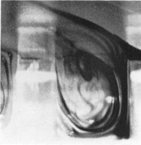
FIG. 6. Example of the so-called "strong exchange" phase. Slot size \frac{1}{4} \times \frac{1}{4} in, free stream velocity 0.520 ft/s, \epsilon^* = 49.3 . An idealized sketch is shown on the right.
