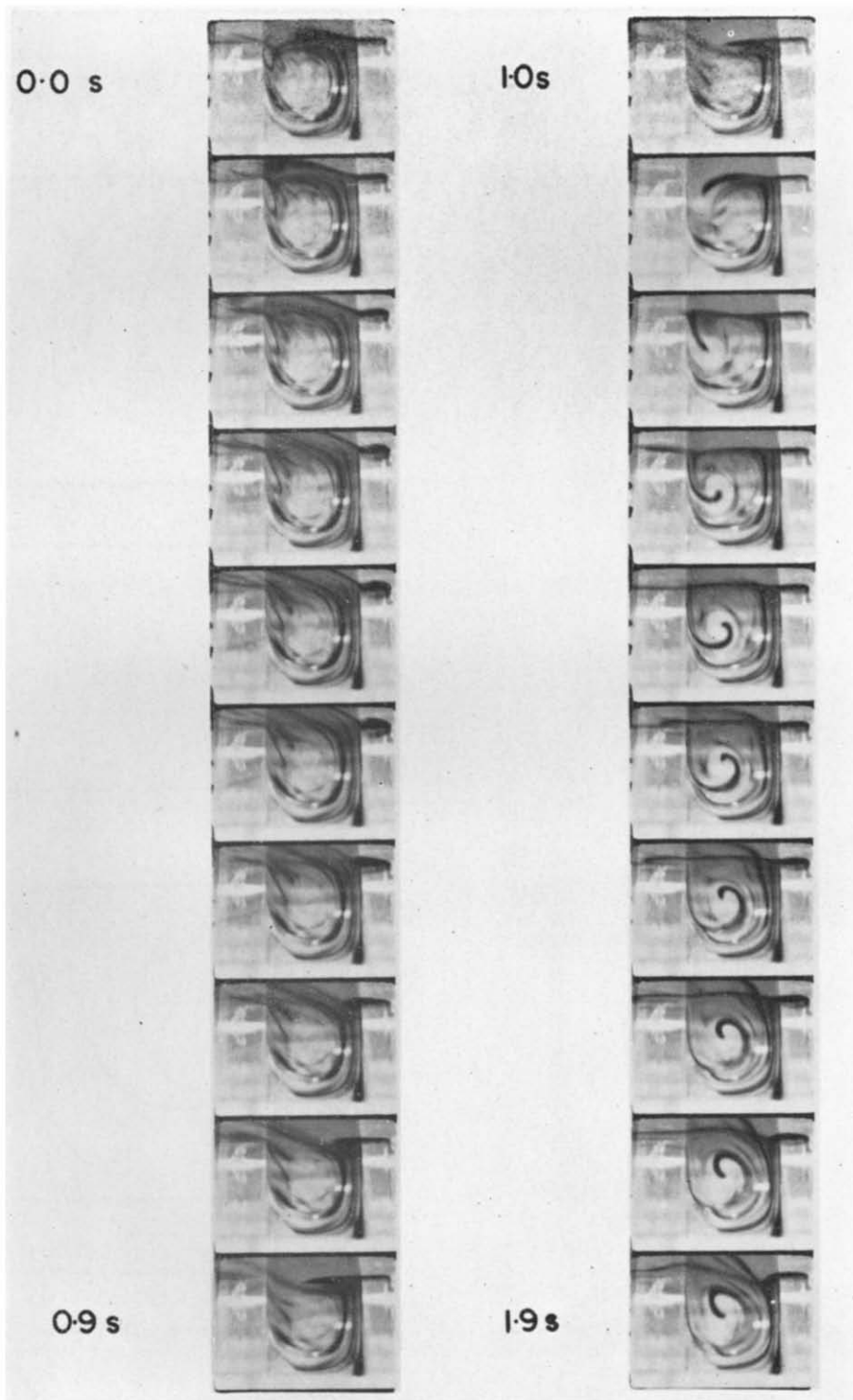
FIG. 10. Series of motion picture frames taken for a period of 2 s at 10 frames per second. Slot size \frac{1}{4} \times \frac{1}{4} in, free stream velocity 0.520 ft/s, \epsilon^* = 49.3 . The series illustrates the unsteady character of the flow and shows several of the flow phases.
